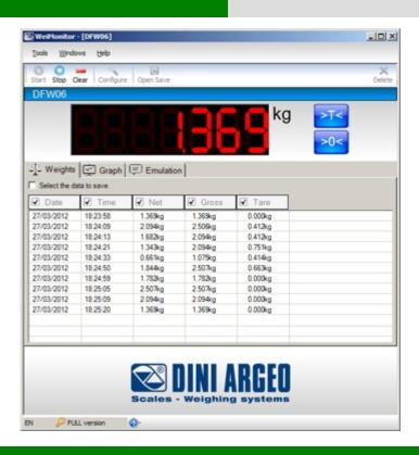
WeiMonitor is the PC program which allows you to monitor and record in real time all the weighings made on the connected scale, storing them in a text or Excel file for further processing.
