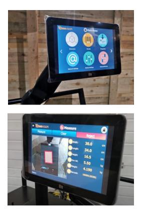
**Resolution 3** is a low cost/high quality dimensioning and weighing system that can calculate dimensions, volume, weight and volumetric/dimensional weight in a fraction of a second.
