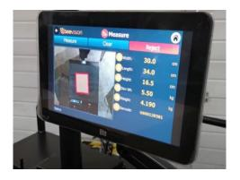
The image capture and dimensioning can be triggered at the press of a button or by scanning a barcode. The dimensions and weight are then calculated in an incredible 0.05 seconds. The data and image is stored and optionally sent via Ethernet, RS232 serial or Wifi to a server or 3rd party software. Configuration and integration is easy using the web interface and our powerful and simple to use API.
