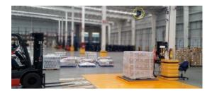
The image capture and dimensioning can be triggered at the press of a button or by scanning a barcode. The dimensions and weight are then calculated in an incredible 0.05 seconds. The data and image is stored and optionally sent via Ethernet, RS232 serial or Wifi to a server or 3rd party software.
