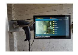
The image capture and dimensioning can be triggered at the press of a button or by scanning a barcode. The dimensions and weight are then calculated in an incredible 0.05 seconds. The data and image is stored and optionally sent via Ethernet, RS232 serial or Wifi to a server or 3rd party software. Configuration and integration is easy using the web interface and our powerful and simple to use API.
