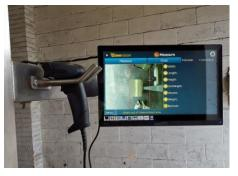
The system uses the powerful Resolution One Dimensioning Camera which can operate stand alone or can seamlessly connect to a weighing scale for weight and dimensions.
