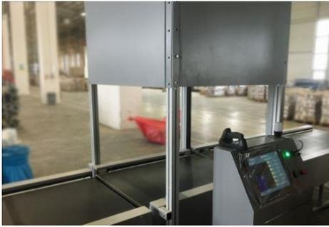
Barcodes are automatically scanned and images stored in the Resolution Five indicator for viewing on the screen or sending to a PC. A separate handheld barcode scanner supplied for damaged or inaccessible barcodes. The system stops to allow unreadable barcodes to be entered and then continues to process parcels, pausing to allow correct spacing between items for perfect dimensioning performance.
