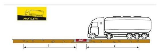
This reinforced ale weigher allows you to calculate the weight of a vehicle in transit, summing the various axles, weighed dynamically or statically. Designed for flush/pit installation and calibrated to a variety of weight displays to suit your specific application.
